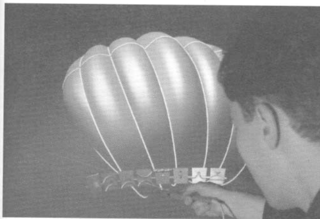
Figure 1: 3D styling of surfaces on the Responsive Workbench (RWB) TM
