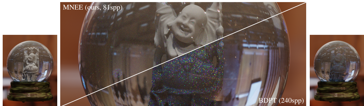
Figure 1: A Stanford Buddha in a glass sphere showcasing the robustness of our method in the presence of refractive caustics. Our technique can efficiently sample this transport: the two images are an equal time comparison of our method to bidirectional path tracing. While the raw speed impact is about 3\times , an equal quality comparison would render our method many thousand times more efficient here.
